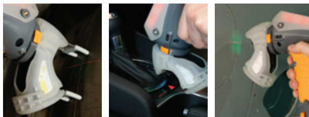
Reglaj raza laser intrerupta, raza laser scurta, raza laser lunga.
